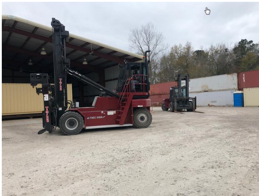
Figure 4-7 – Container top loader and mid-sized forklift
